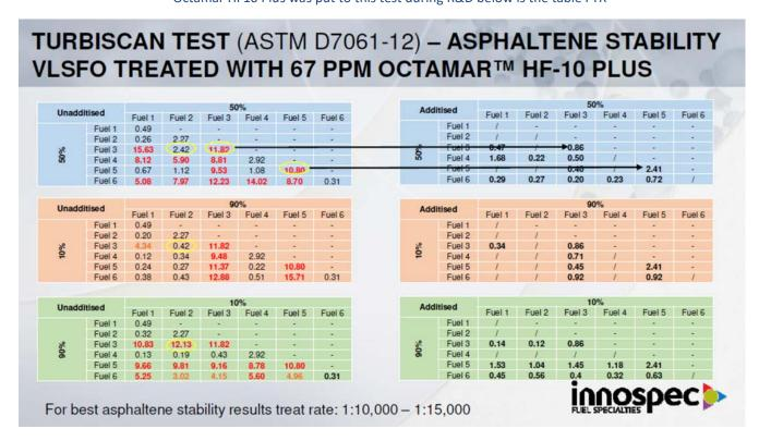
Table on left indicates the fuel mixing at various ratios (10-90, 50-50 & 90-10) and not treated with chemicals. Those mixing with RSN result indicated in Red(over 5) is bad or unstable.
