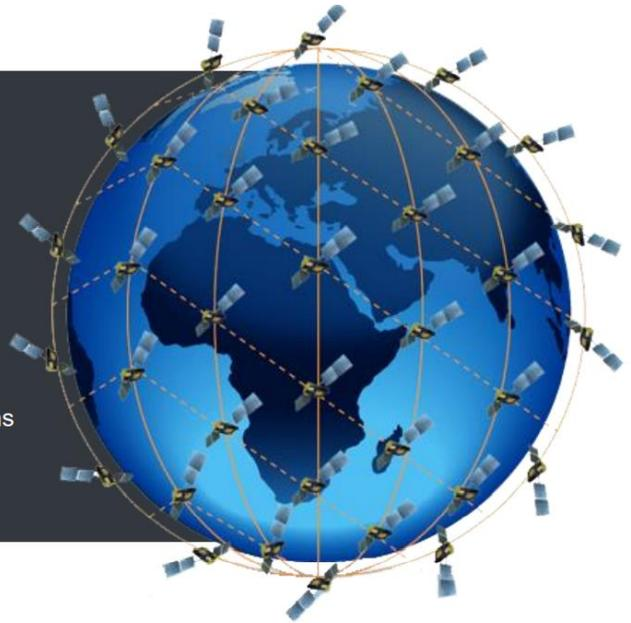
Iridium Certus runs on high-speed L-Band. L-Band is the lowest frequency commonly available for maritime satellite communications, meaning that the Iridium signal can penetrate clouds, fog, and rain better than higher frequency Ka- and Ku- band signals.
